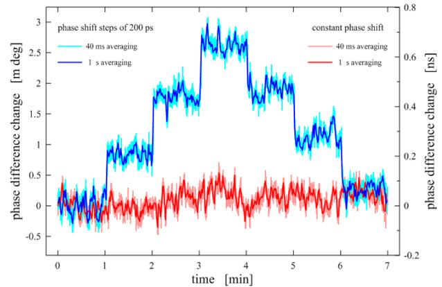
Figure 7: Response of the differential phase detector upon 200 ps delay steps (in cyan and blue) and the detector 7 minute stability (in red).
