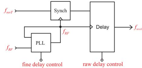
Figure 4: Programmable Delay Line (PDL). Abbreviations: Sync – synchronisation circuit.
