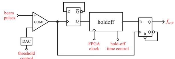
Figure 3: Block diagram of the Local Timing Generator (LTG).
