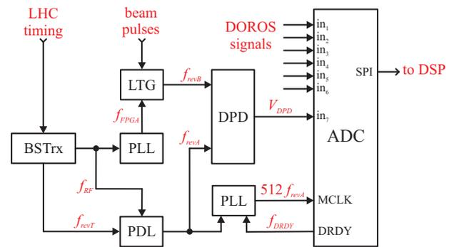
Figure 2: DOROS synchronisation circuits. BSTrx – beam synchronous timing receiver, LTG – local timing generator, PDL – programmable delay line, DPD – differential phase detector, MCLK – master clock, DRDY – data ready signal.
