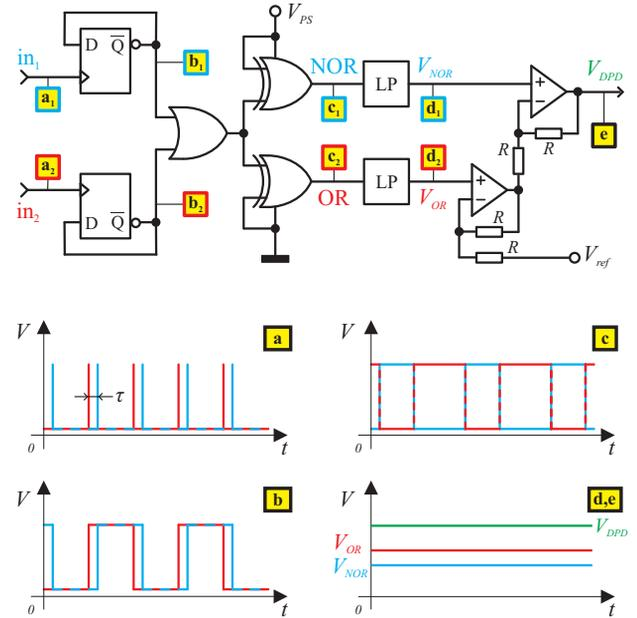
Figure 5: Block diagram of the Differential Phase Detector (DPD) and simplified waveforms in its key nodes. LP – low pass filter.
