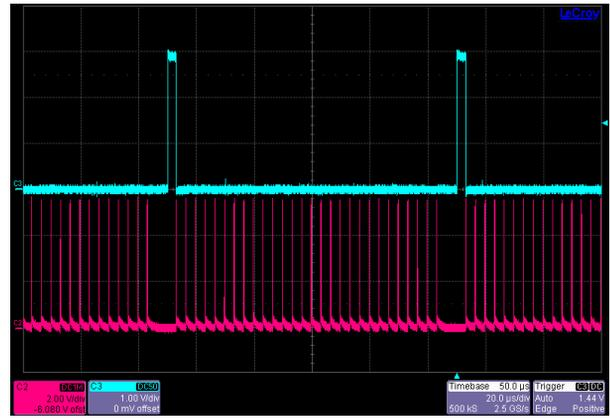
Figure 6: Laboratory testing of the local timing generator (LTG). Shown are the input and holdoff output waveforms in magenta and blue, respectively.
