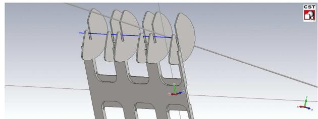
Figure 5: The details of the target frame fins. The shape is designed to have smooth curvature and enough clearance in the chamber. The half elliptical shape allows it to be mounted on every target, but a full elliptical shape should reduce the electric fields further.
