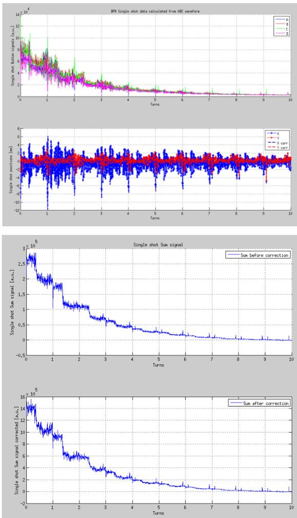
Figure 4: Beam circulating the storage ring for several turns, first turn trajectories and SUM signal from ADC data. There are 180 BPM data points in one turn. (top) four button signals and calculated x/y positions; (bottom) BPM SUM signal before and after corrections.
