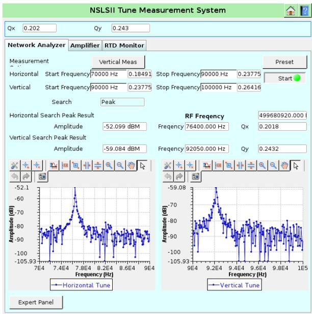
Figure 11: Storage ring sweep tune measurement system operational panel showing the x/y tune spectrums.
