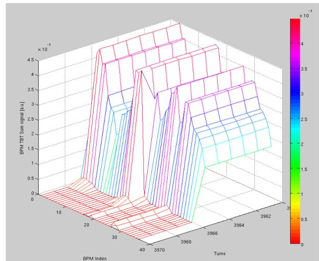
Figure 3: Booster BPM 4-button SUM signal in TbT mode. (top) Beam was injected on TbT sample #4, which is the first turn in Booster. All Booster BPMs saw the beam at same turn. (bottom) Beam was extracted on turn sample #3966 (Offseted by 719236 turns), only the first 18 BPMs saw beam on that turn.
