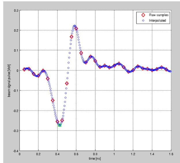
Figure 8: Storage ring filling pattern monitor signal from 20GHz real time sampling scope. Red diamonds were raw sample data points while blue circles were interpolated points by a factor of 10. Green Square is the searched peak of interpolated point, its amplitude was considered to be bunch current and its position was measured synchronous phase.
