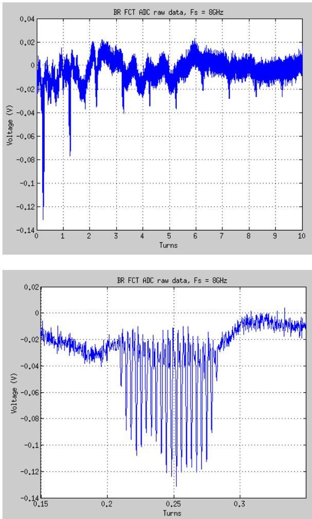
Figure 7: Booster FCT measurements shown beam was circulating for multi-turns (top). 20 bunches were detectable from 8GHz sample rate data (bottom).
