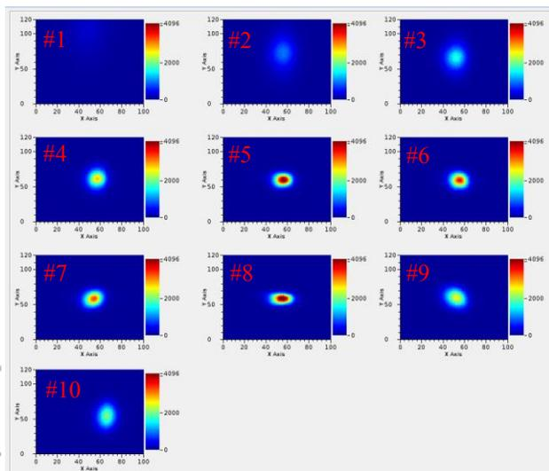
Figure 10: Booster A1 SLM ten burst images during energy ramp. The images were acquired with separation of 40ms.
