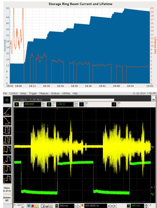
Figure 1: (top) storage ring DCCT measured current and lifetime history plot when fill up to 50mA; (bottom) filling pattern at around 50mA.
