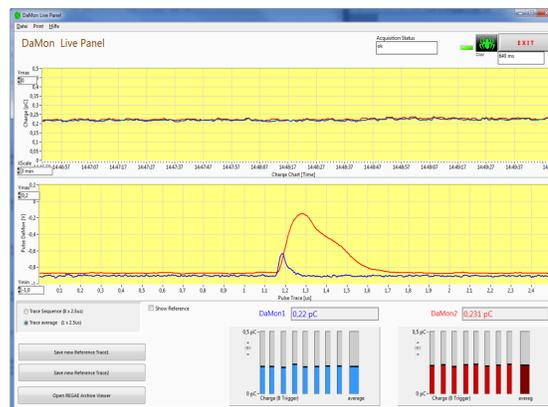
Figure 5a: Graphical User Interface of the DaMon output. Top diagram: a history of the charge values for few minutes; lower diagram: recent voltage as a function of time of both channels with blue the first channel and red the second channel; below: recent calculated charges for last 8 bunches of both channels with the same color definition including a charge average at about 230 fC.
