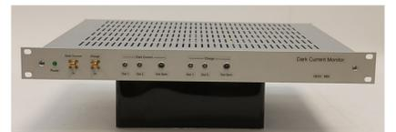
Figure 4: Photo of the DaMon electronics. From left: power control LED, dark current input, beam charge input, 3 dark current outputs (2 times single ended and 1 differential), 3 beam charge outputs.
