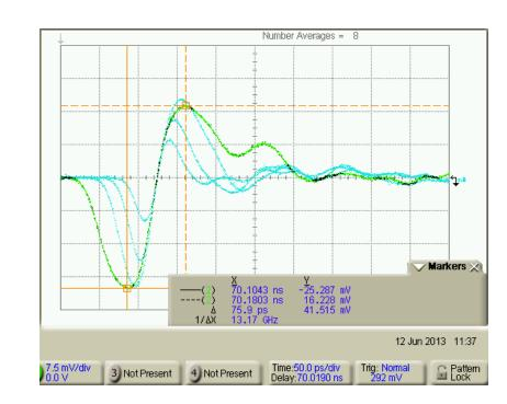
>The flat electrode steepness is 1.35, the button electrode steepness is 0.71, the ratio is 1.9.
