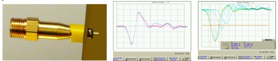
TE-like wave packet converts to TEM-output at the connection point. We didn't try to find an optimal tradeoff of the impedances to get the output maximised. This can be better done using a simulation package.
