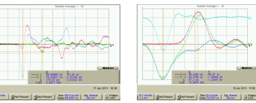
1. The incident packets are spaced by gap length over c. 2.Reflected and passed packets are seen on the right from the grid central line. They are spaced by gap length over c and go in the gaps in **reverse** orders. 3.One more effect is seen: spreading of the incident packet around the electrode into the opposite gap.
