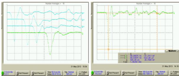
Figure 4: Left: Propagation of a short pulse along the ‘beam’ line, 50ps/div and 7.5mV/div. Right: Back response of a long gap, 100ps/div and 5mV/div.
