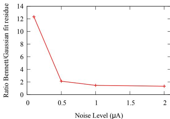
Figure 5: Ratio of the residue from Bennett and Gaussian fits from simulated Gaussian beam data with  $\sigma = 8$  mm, displacement  $z = 5$  mm and beam current  $I_{beam} = 150 \mu\text{A}$ . At low noise levels it is easy to tell that the data comes from a Gaussian beam as the residue from the Bennett fit is far higher.
