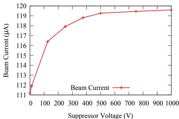
Figure 2: Relation between the applied suppressor voltage and the measured beam current. Without suppression one secondary electron for every ten  $H^-$  leaves the cup and falsifies the measurement. 500 V are sufficient to suppress most of this effect.
