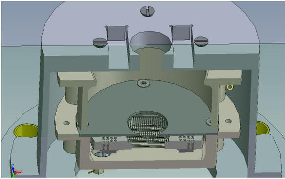
Figure 1: The Faraday Cup with the integrated Wire Grid.
