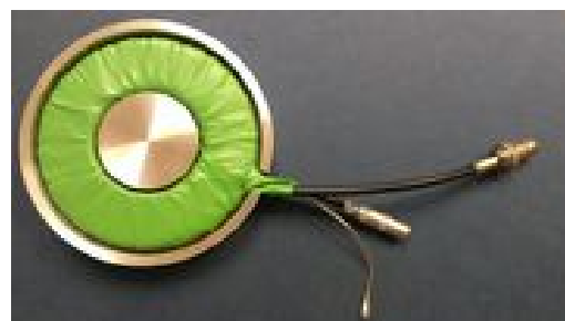
Figure 2: In-house designed and built toroid.
