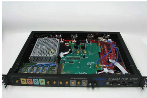
Figure 3: BPM signal processing electronics with the top cover removed.
