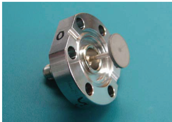
Figure 2: The button electrode for beam position measurements.
