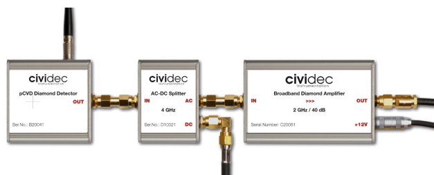
Figure 1: Diamond Beam Loss Monitor.
