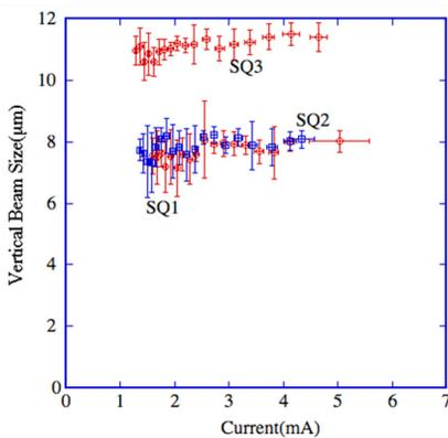
Figure 16: Results of X-Y coupling tuning by using the conventional refractive SR interferometer with the skew Q at ATF.
