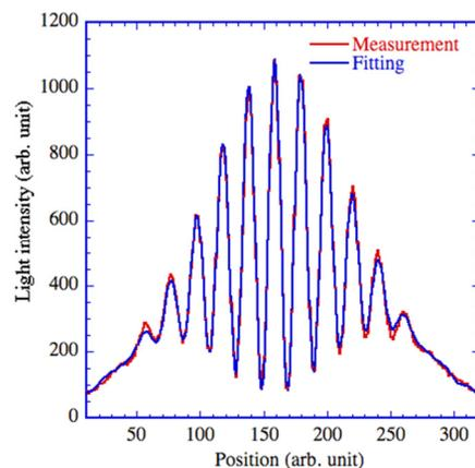
Figure 14: Measurement result of interferogram at KEK ATF Dumping ring with an interferometer having an off-axis Herschelian optics. Red line is measurement result, and blue line is result of best fitting.
