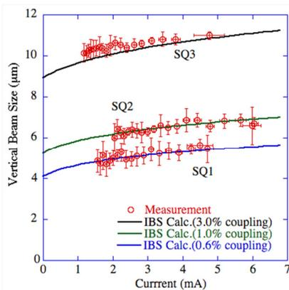
Figure 15: Result of X-Y coupling tuning by using the off-axis Herschelian SR interferometer with the skew Q at ATF.
