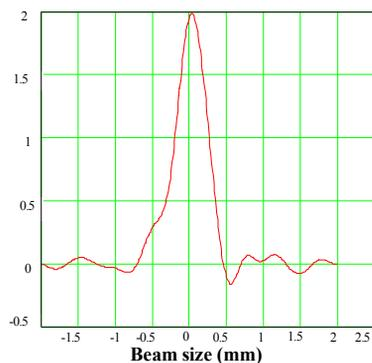
Figure 6: Reconstructed vertical beam profile by Fourier inverse transform of complex degree of 1<sup>st</sup> order spatial coherence.
