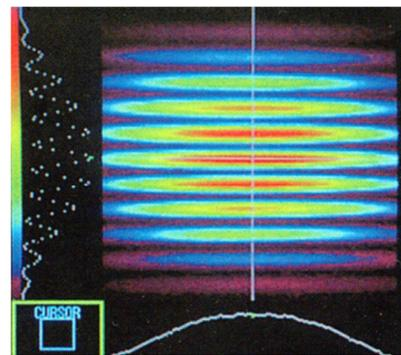
Figure 3: A typical interferogram observed with the SR interferometer.
