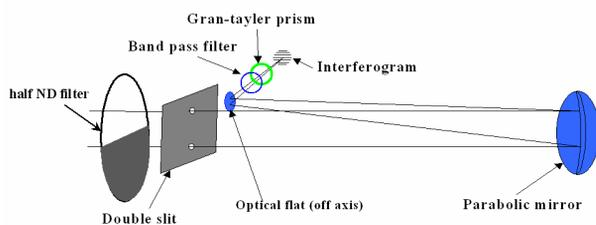
Figure 24: Setup of imbalance input interferometer. A special ND filter which lower half of glass flat is covered with an Aluminium coating is set in front of double slit.
