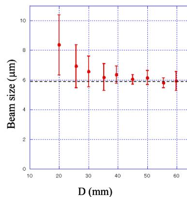
Figure 17: Increase of the beam size in small separation range of double slit.  $D=40\text{mm}$  corresponds to  $\gamma=0.924$ .
