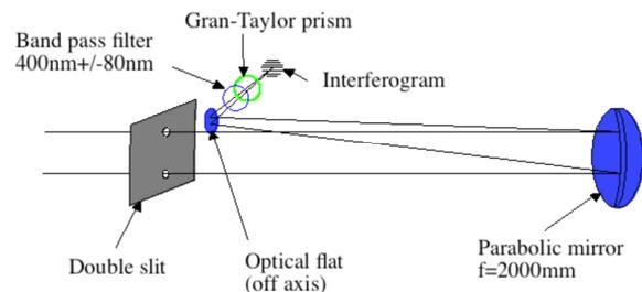
Figure 13: An off axis Herschelian arrangement applied for double slit interferometer.
