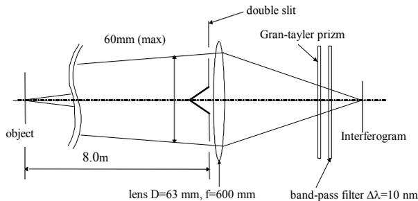
Figure 2: Outline of the SR interferometer. The wavefront-division type of two-beam interferometer.
