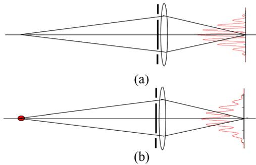
Figure 1: A simple representation of the visibility of an interferogram and light source size. (a) A point source yields an interferogram with a visibility of 1; (b) an ensemble of point sources yields a reduced visibility.
