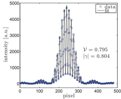
Figure 9: Interferogram with the skew quadrupoles off.
