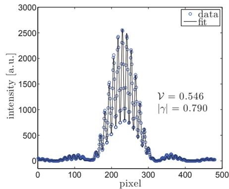
Figure 10: Interferogram taken with the intensity imbalanced interferometer with the skew quadrupoles turned off.
