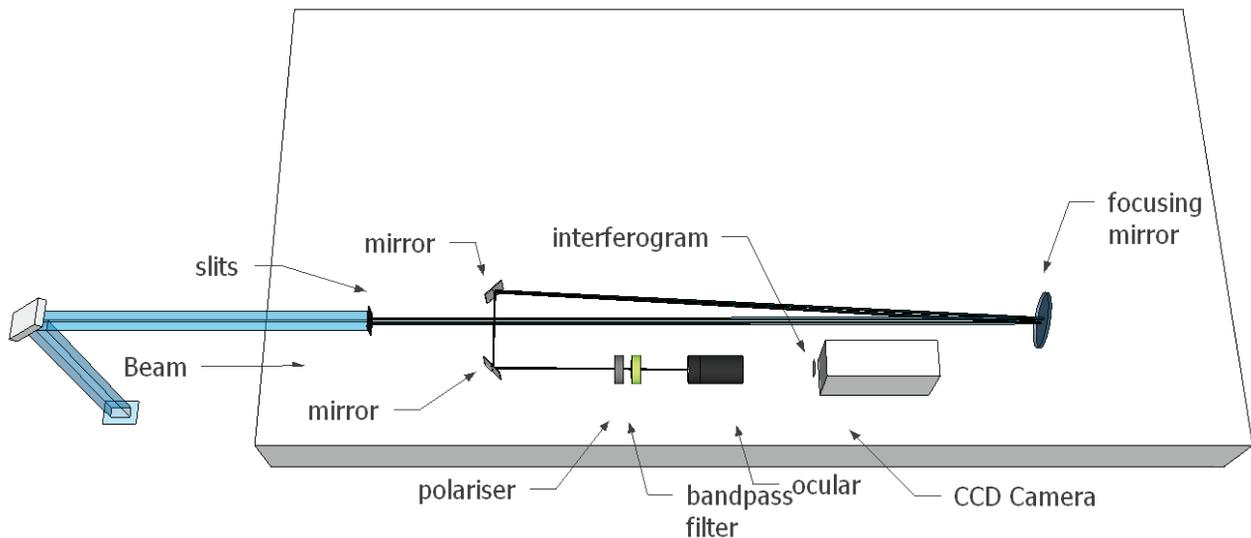
Figure 3: The currently used configuration of the Mitsubishi apparatus interferometer as used at the ATF2 at KEK (March 2012).
