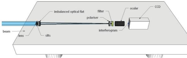
Figure 8: The refractive optics setup of the intensity imbalanced interferometer on the optical diagnostic beamline at the Australian Synchrotron.
