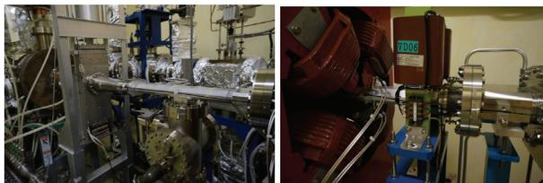
Figure 4: Black cables mounted on the side of the vacuum chamber are the optical fibers for the loss monitor. The fibers can be fed through the magnet due to the non-magnetic nature of the medium.
