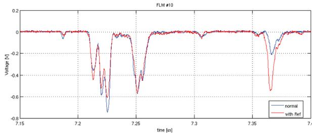
Figure 3: Signal without (blue) and with (red) reflector.
