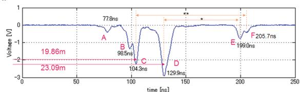
Figure 2: Determination of loss location.
