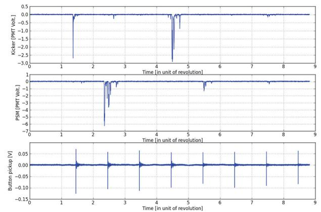
Figure 7: Beam loss measured using two injection systems: kicker magnets (top) and a pulsed sextupole magnet (middle). The bottom figure shows the signal from a button pickup electrode near the vertical wiggler. No beam is stored in the ring prior to injection. The horizontal axis represents the turn number, namely, time in unit of revolution of the PF-Ring.
