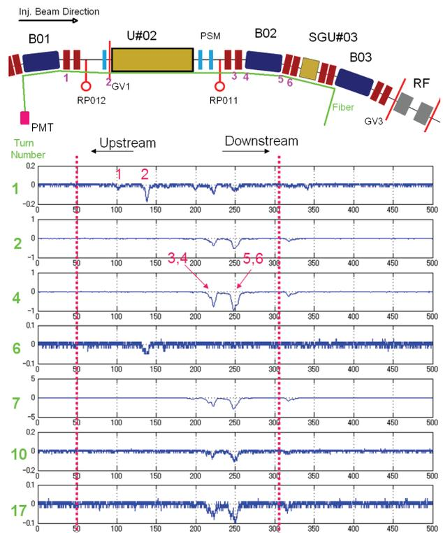
Figure 5: Layout of storage ring components and optical fibers (top) and detected loss signal (bottom) on each turn. The electron beam travels from left to right in the figure.
