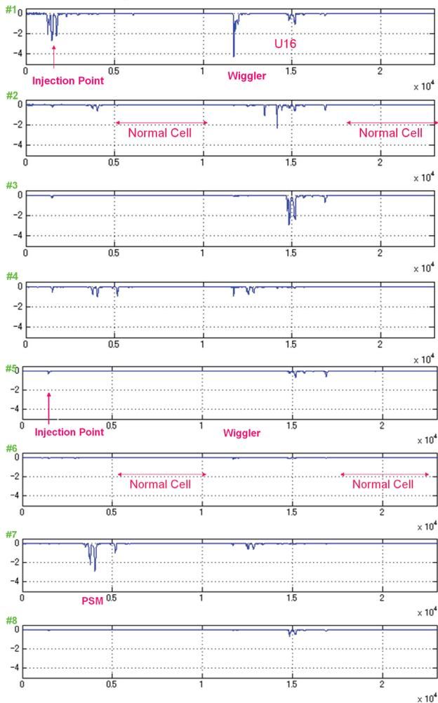
Figure 6: Beam loss over the whole ring. In each row, the horizontal full scale corresponds to the entire ring circumference of 187 m.
