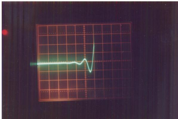
Figure 2: Photograph of induced pulse from induction monitor.
