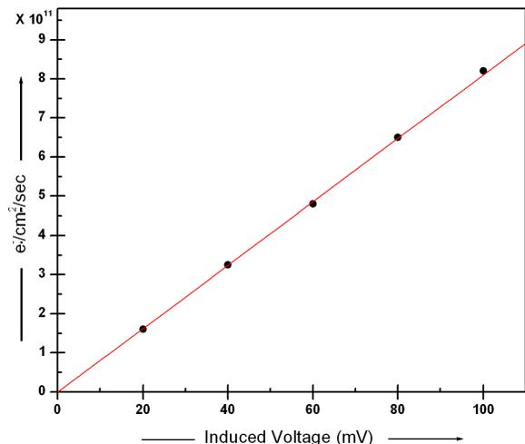
Figure 4: Calibration curve for the induced current monitor.
