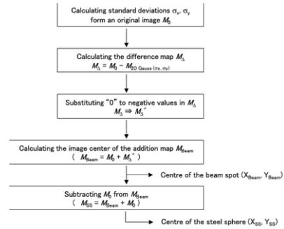
Figure 5: Algorithm to calculate the beam misalignment.
