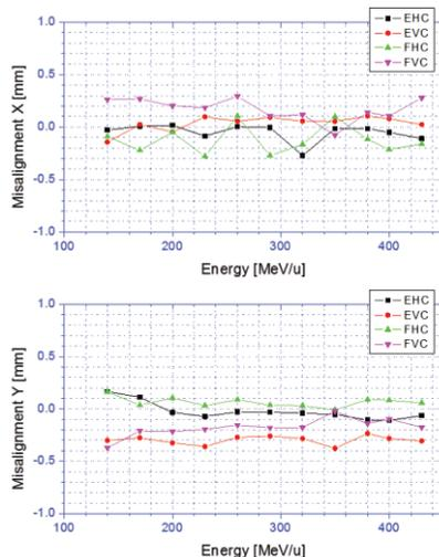
Figure 8: Measurement results of the beam misalignment.
