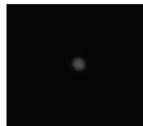
Figure 2: Typical image of the beam spot measured by the 2D beam imaging system.
