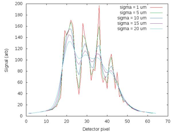
Figure 4: Simulation of expected beam patterns for 50-micron pitch detector at different beam sizes.
