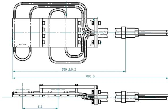
Figure 2: The construction of two Be mirrors.
