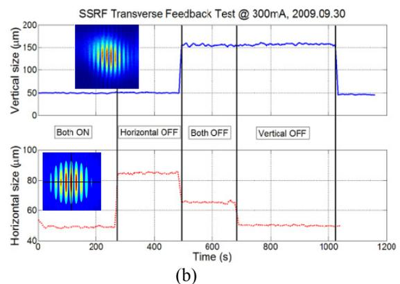
Figure 4: (a) the interferogram and beam image variation for feedback on or off; (b) X and Y beam size variation for feedback on or off.
