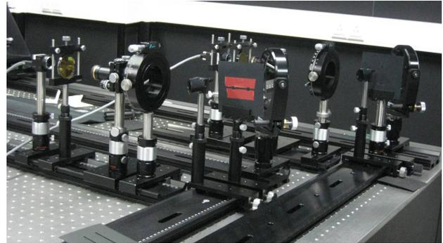
Figure 3: Arrangement of SR interferometers.
