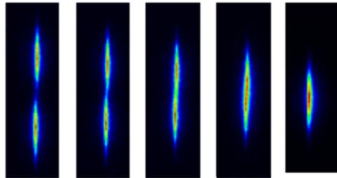
Figure 6: The drifting between bunches while beam injection.
