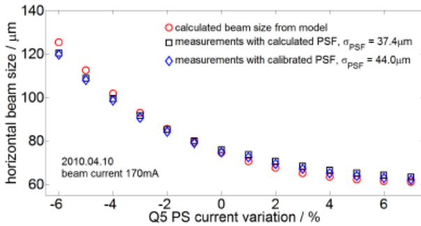
Figure 5: Comparison of calculated beam size and measured beam size.
