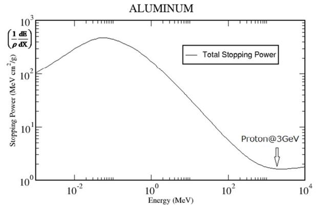
Figure 4: Stopping-power estimated for protons in aluminium.
