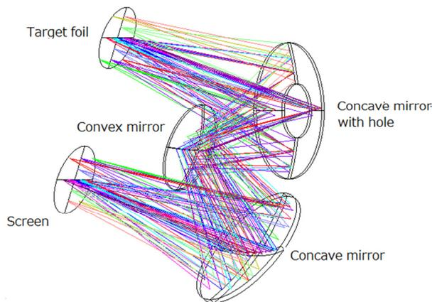
Figure 6: Offner relay system for large aperture.
