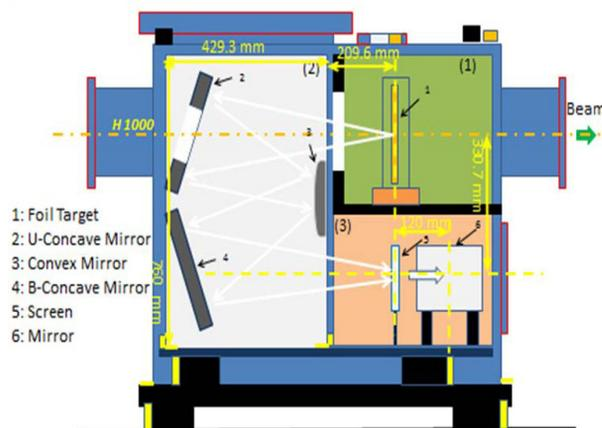
Figure 9: Schematic of the OTR monitor at 3-50BT.
