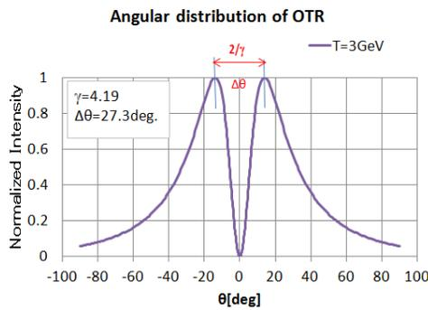
Figure 2: The angular distribution of OTR emitted from 3 GeV ( $\gamma=4.2$ ) proton beam.
