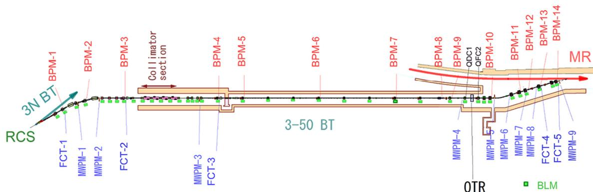
Figure 1: A schematic drawing for layout of beam instrumentations for 3-50BT in J-PARC. New beam profile monitor using the OTR is planned to set between QDC1 and QFC2. The collimator section locates between BPM3 and BPM4.
