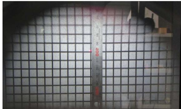
Figure 10: Test of grid pattern for Offner relay system. Grid spacing is 10 mm.
