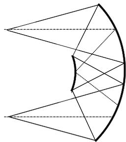
Figure 5: Schematic drawing of Offner optical system.
