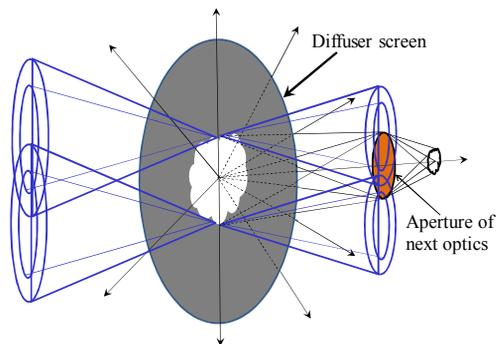
Figure 11: Diffuser screen to convert the angular distribution of OTR into uniform illumination for next optics.
