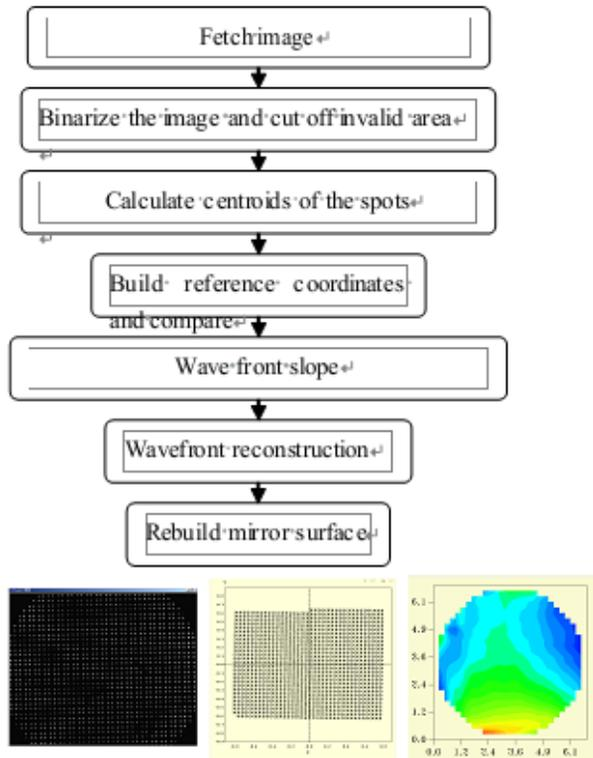
Figure 7: Data process flow of Shack-Hartmann screen test.
