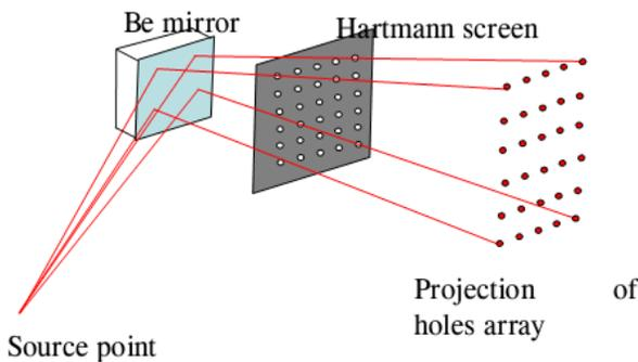
Figure 4: Hartmann screen to measure mirror deformation.
