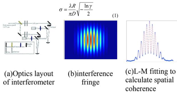
Figure 2: Measurement of beam size.
