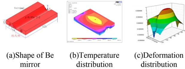
Figure 1: Design and simulation of the Be mirror.
