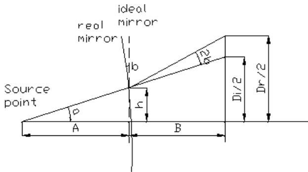
Figure 3: Deformation of mirror influence to D(separation of double slits).
