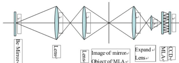
Figure 6: Optical layout of Shack-Hartmann screen test.
