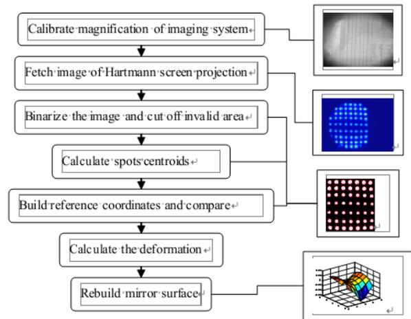
Figure 5: Data process flow of Hartmann screen test.
