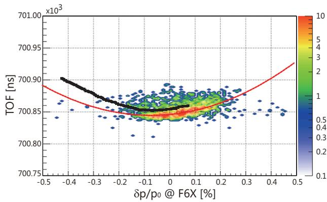
Figure 3: Revolution time as a function of the momentum of  $^{78}\text{Kr}$  ions. Red curve is a fitted curve of the 2nd order polynomial. Black curve was obtained from the Schottky data after the conversion of the resonance frequency into the revolution time and the time after injection into the momentum based on the energy loss calculations in residual gas in the ring.
