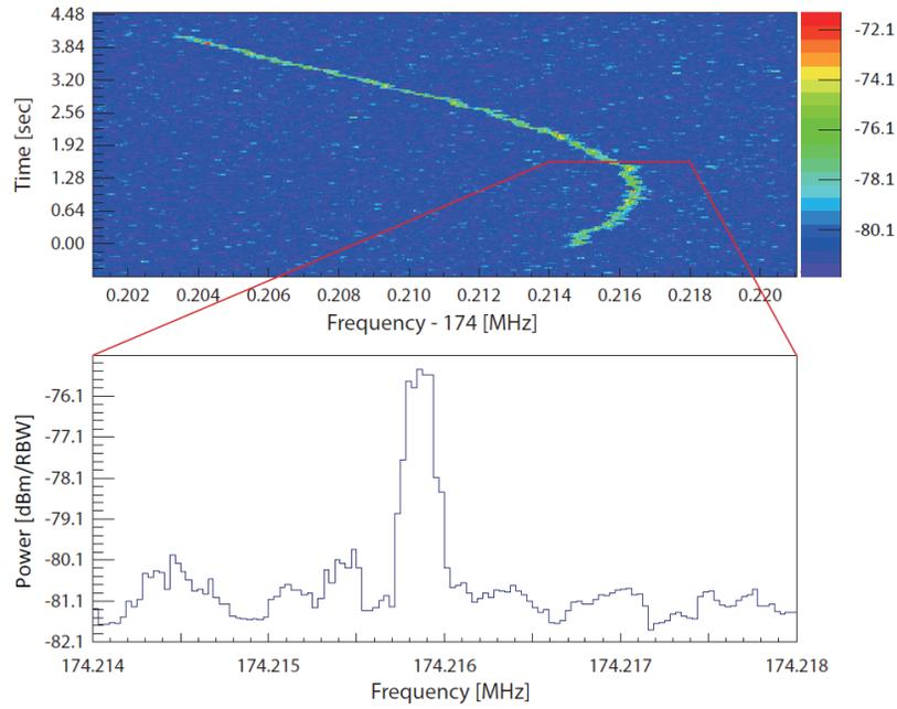
Figure 2: The upper part is a spectrogram of a single  $^{78}\text{Kr}$  ion. The  $^{78}\text{Kr}$  ion was stored for 4 s. The lower part is a zoomed FFT spectrum in a frame of 32 ms. The output signal power is  $P = -65.8$  dBm which is obtained by integrating the peak after subtracting the thermal noise. The frequency width is 224 Hz in FWHM.
