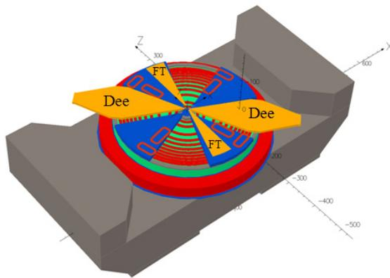
Figure 2: The model of DC-280 magnetic system.
