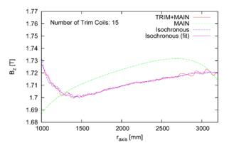
Figure 4: Vertical field  $B_z$  along X axis (see Figure 3). TRIM+MAIN: Field generated by main coil and trim coils by optimized parameters. MAIN: Field generated by main coil alone. Isochronous: Isochronous field shown in Formula using raw  $K_B$ ,  $K_r$ . Isochronous (fit): Isochronous field using  $K_B$ ,  $K_r$  fit by quintic curves.
