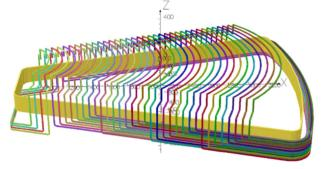
Figure 3: HTS main coil and 36 trim coils on one pole of sector magnet. Main coil size is 2.8 m along X axis.
