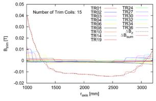
Figure 6: Excitation level of 15 trim coils to fit  $\Delta B_z$ .
