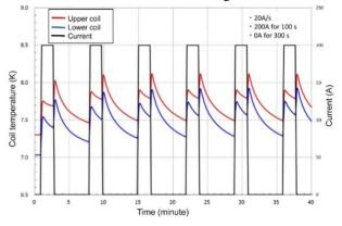
Figure 9: Coil temperature during ramping operation. Ramping rate is 20 A/s.
