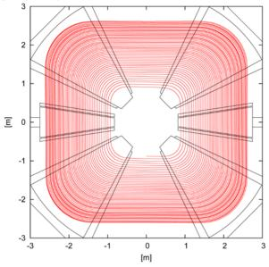
Figure 7: Orbit simulation on isochronous field.
