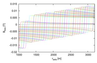
Figure 5: Contributions on vertical field by 36 trim coils excited to 504 A. Trim coils are exited one by one on main field and subtracted main coil contribution.
