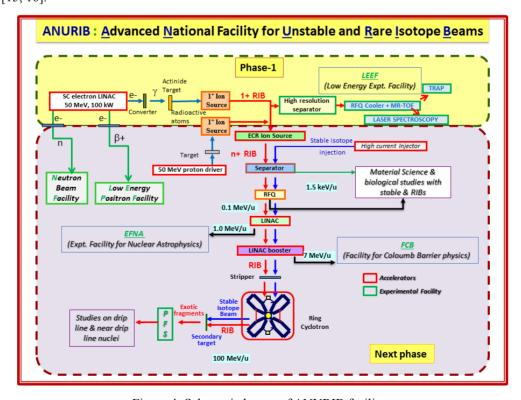
Figure 4: Schematic layout of ANURIB facility.
