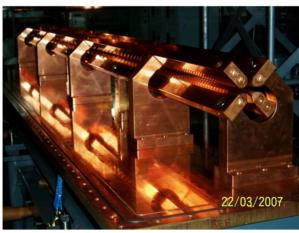
Figure 2: Photograph of the internal post-vane structure of 3.4 m long RFQ linac taken during installation at VECC.
