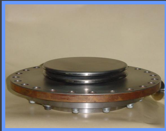
Mechanical tuner (Nb)
