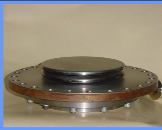
Mechanical tuner (Nb)
