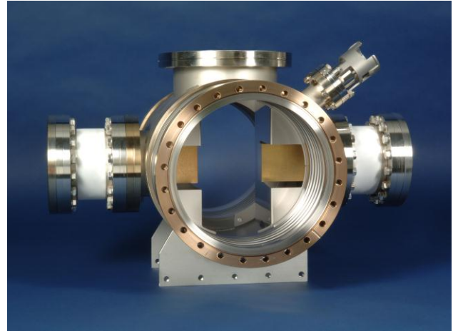
Fig. 11: NEG coated scraper chamber with Au coated Cu ion catcher blocks. Diagnostics: extractor ion gauge and current measurement of charge exchanged ions.
