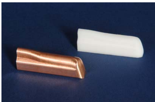
Figure 15. Plastic model (GSI construction department) and copper test piece of the RFQ Input Radial Matcher (NTG Neue Technologien GmbH).
