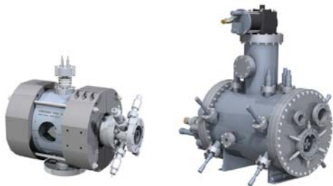
Figure 1: 3D Drawing of the Dresden EBIS-A (left) and the Dresden EBIS-SC (right). In each case the ion extraction can be seen on the right.
