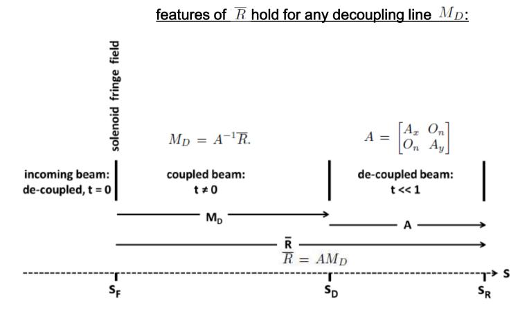
•  $\overline{R}$  has the decoupling features
