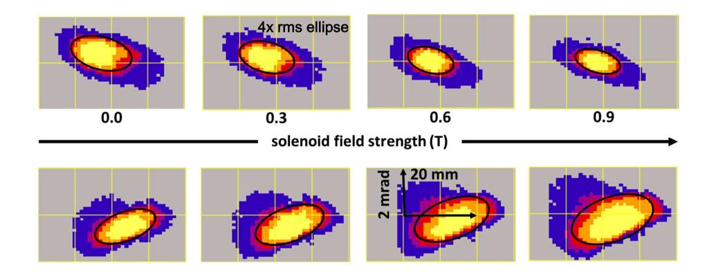
Twiss parameters beta & alpha in both planes remain constant within resolution of measurement
