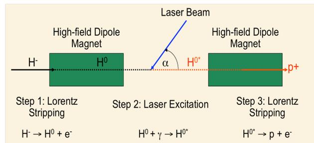
Figure 1: The laser stripping concept.
