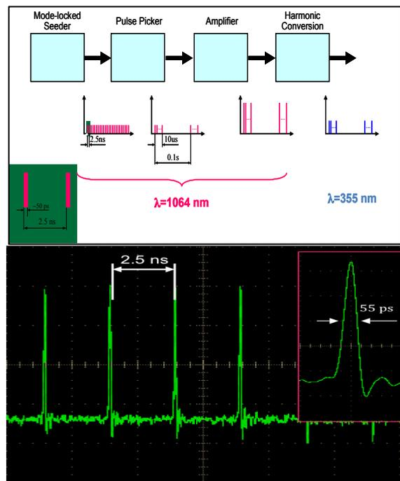
Figure 3: (Top) Laser amplification scheme. (Bottom) Laser microstructure measurement.
