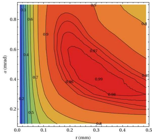
Figure 5: Simulated laser stripping efficiency versus laser radius and divergence.
