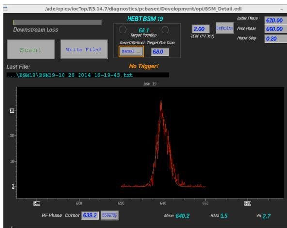
Figure 4: BSM measurement of a 22 ps microbunch.
