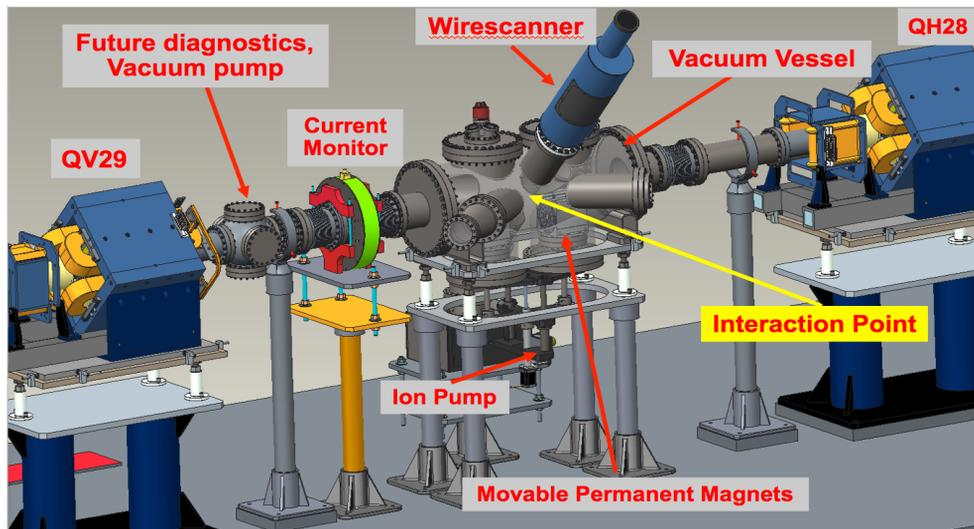
Figure 2: The final design of the experimental station.
