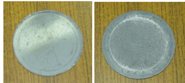
Figure 5: The vacuum side (left) and water side (right) of the Beryllium target.
