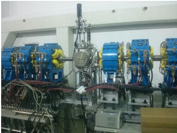
Figure 10: 2D beam profile measurement system.
