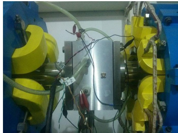
Figure 15: The button-type BPM on the beam line.
