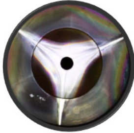
Figure 8: Plasma bombardment images on plasma electrode.
