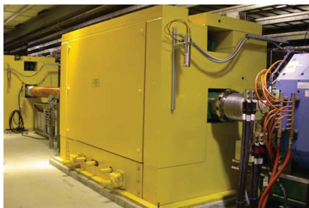
Figure 7: SNS multi-layered collimators, each designed to withstand 10 kW protons at 1 GeV.
