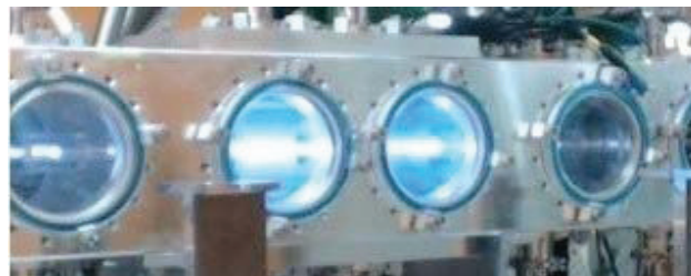
Figure 5: Test of He gas charge stripper using Uranium beams at RIKEN [39].
