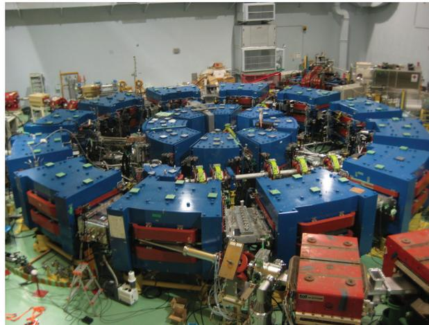
Figure 1: The KURRI 150 MeV FFAG is the larger ring shown here with the pre-2011 injector ring. Injection from the new linac occurs in the top left of the image.
