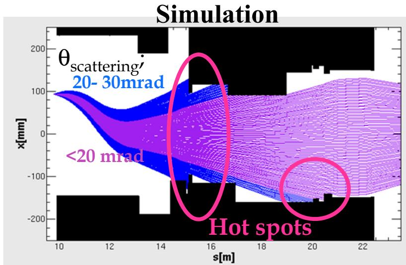
Install absorber to catch a foil scattered particles into hot spots (A)
