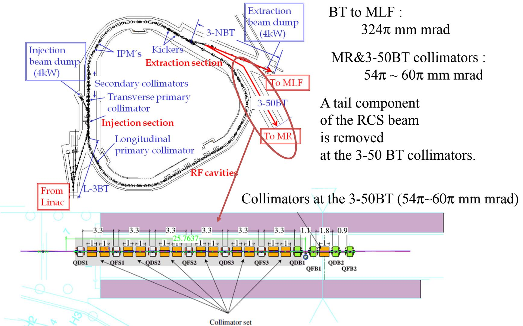
The first matter for the MR injection is to pass the high intensity beam through the 3-50BT collimator within the permissible beam loss level (<2 kW).
