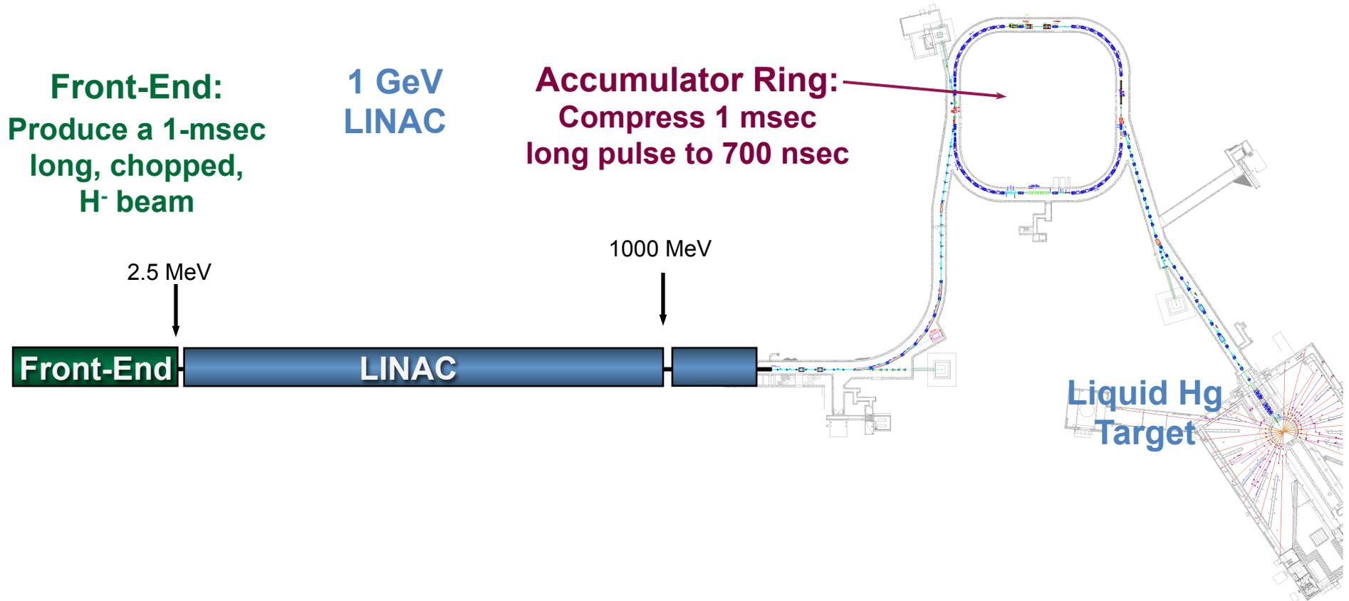
Approximately 365 beam loss monitors cover the linac, ring, and transport beam lines
