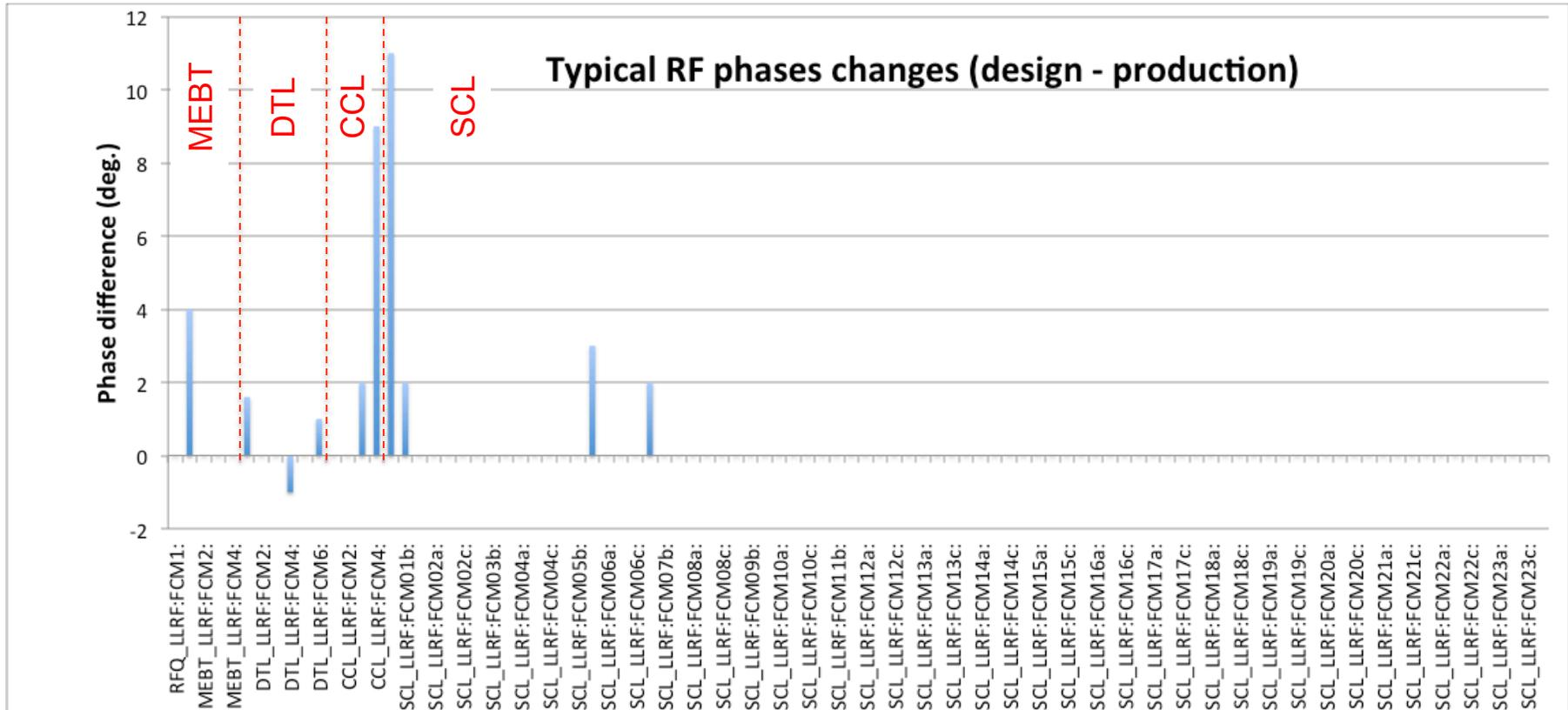
Some RF phases must be empirically adjusted to achieve the low-loss tune
