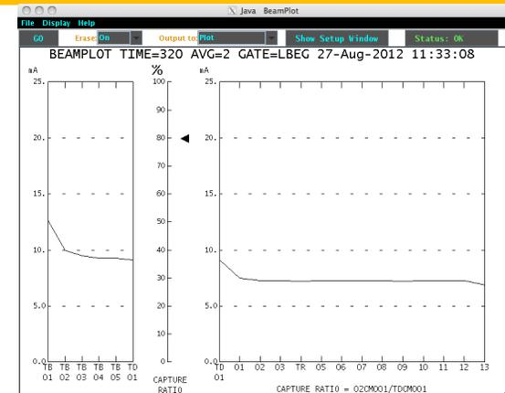
Current Monitors along H<sup>-</sup> LEBT, DTL and portion of CCL showing capture losses in DTL
