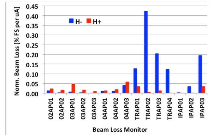
Comparison of H<sup>+</sup> and H<sup>-</sup> beam loss normalized to current in the vicinity of the TR.
