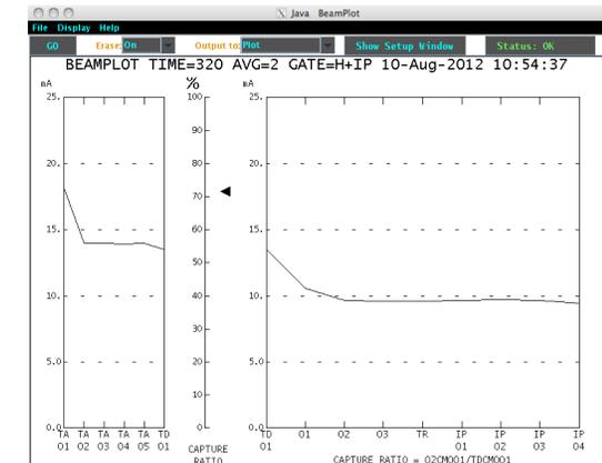
Current Monitors along H<sup>+</sup> LEBT, DTL and IPF beam transports showing capture losses in DTL
