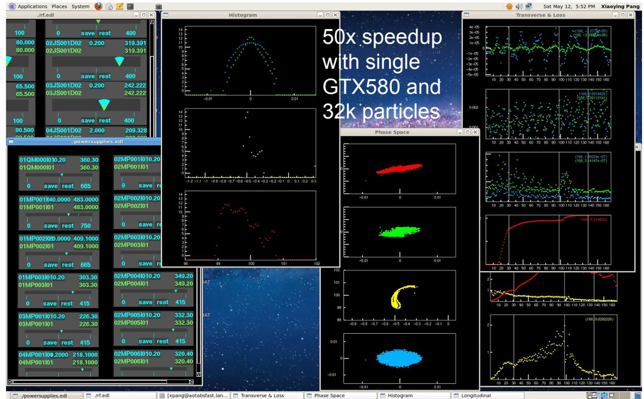
Screen image of High Performance Simulator generated beam profiles and phase-space distributions(center) at end of DTL. Also shown are EPICS DTL RF and magnet controls (left) and beam centroid, size, loss and emittance profiles (right).
