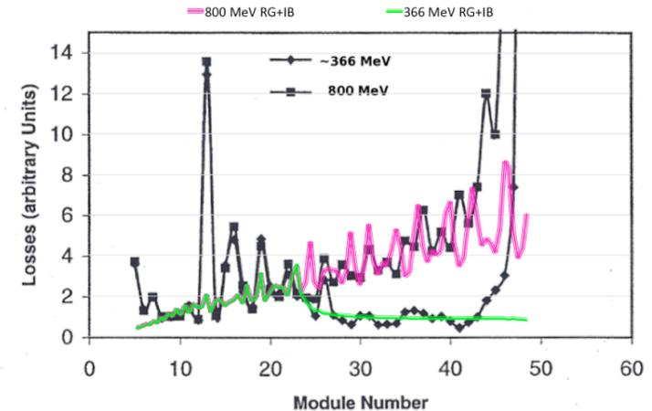
Comparison of measured and simulated beam loss profiles for 366 and 800 MeV H<sup>-</sup> beam. [6] Relative contribution: IB≈75%, RG≈25%
