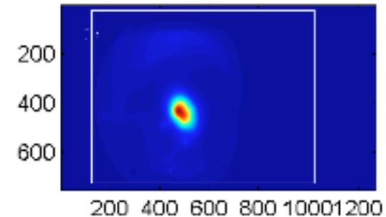
Image plate exposed to CCL-only source of high-energy H<sup>+</sup>. Color indicates intensity.
