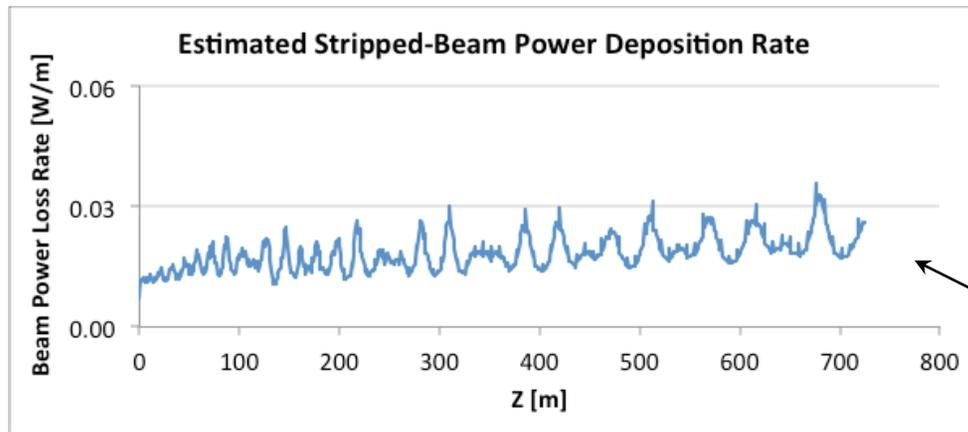
**Few 10's mW/m of stripped beam power loss in CCL**
