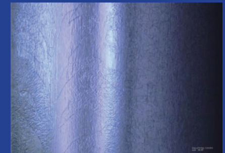
After CBP and 40 microns EP – Pit completely removed
