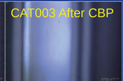
After CBP and 40 microns EP – Pit completely removed
