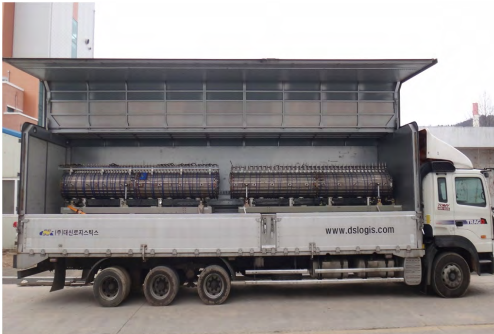
DTL tanks inside vibration free truck
