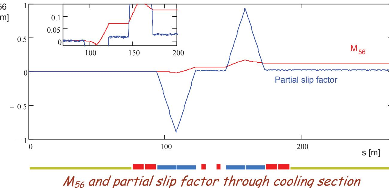
High accuracy of beam optics control is required to prevent uncontrolled sample lengthening
