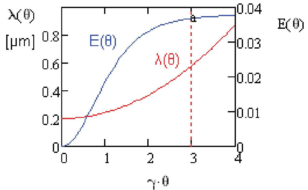
Dependence of the first harmonic wave length on angle (red) and kick strength for a lens with radius determined by subtended angle  $\theta$  ( $a = L\theta$ , blue, arbitrary units)
