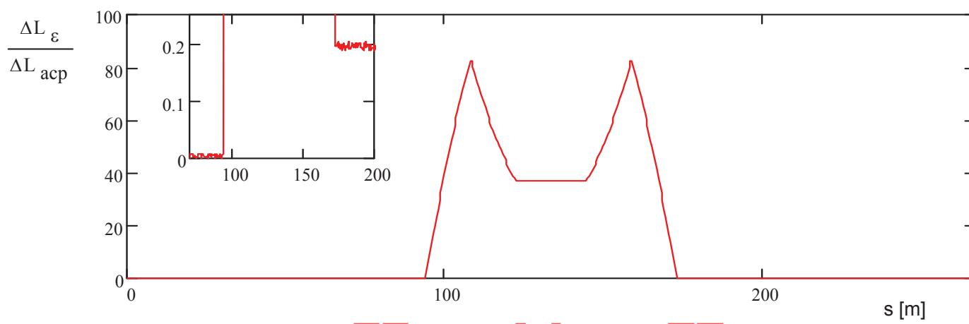
*Ration of sample lengthening due to betatron motion to the transverse cooling acceptance through the cooling section*
