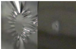
Figure 2: Thin aluminized Kapton target (left) and stainless steel target (right) after irradiation with  $10^{10}$  Uranium ions per pulse. Visible target modifications due to heating-up are observed.
