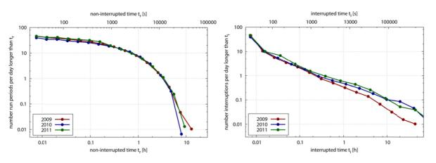
Figure 6: Frequency of uninterrupted run periods per day (left) and interruptions per day (right). The graphs represent histograms that are integrated from long to short time intervals. For example one can read from the left graph that on average 8 uninterrupted run periods per day last longer than one hour.
