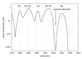
Figure 4: Beam density measured at extraction on a logarithmic scale. The turn numbers are indicated at the peaks.
