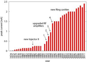
Figure 2: Development of the maximum attainable beam current in the HIPA facility.
