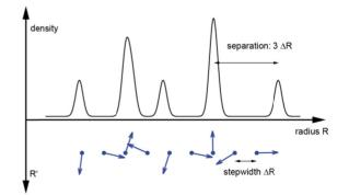
Figure 3: Using eccentric injection, the turn separation at the extraction septum can be maximized. The figure shows radial phase space vectors of the orbit oscillations and the resulting beam density.
