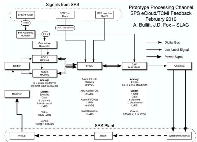
Figure 2: Block diagram of the signal flow for the initial SPS processing testbed system, intended to control a small number of bunches and explore processing algorithms.
