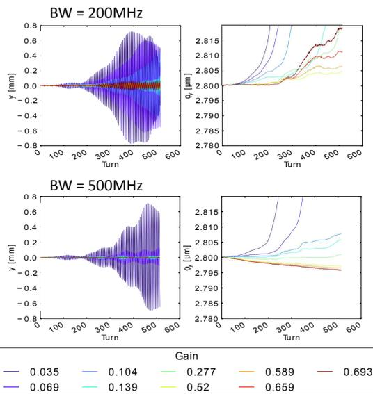
Figure 7: The evolution of the bunch centroid motion and the normalized emittance for different loop gains for kicker  $BW = 200\text{MHz}$  and  $BW = 500\text{MHz}$ .
