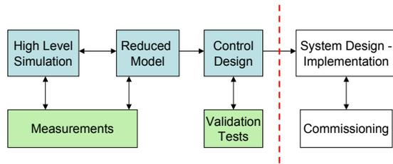
Figure 1: Simplified R & D chart for the development of the broad-band feedback control system.
