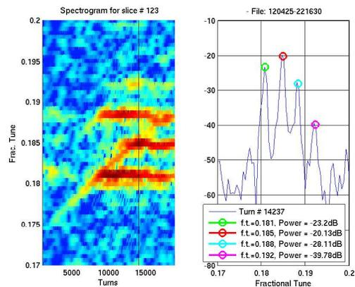
Figure 3: A spectrogram showing excitation of many intrabunch modes for a normalized frequency ( $f/f_{REV}$ ) sweep from 0.175 - 0.188. The betatron frequency is  $f_\beta = 0.181$  and  $f_s \approx 0.004$ .
