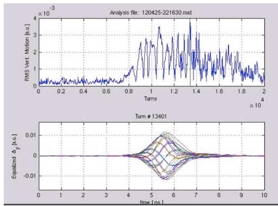
Figure 4: Top: RMS of the vertical motion. Bottom: Equalized delta signal showing multiple modes for turns 13401-13426.
