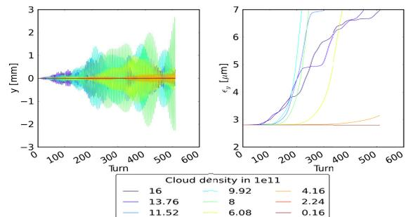
Figure 6: The evolution of the bunch centroid motion and the normalized emittance for different central cloud densities.
