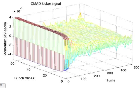
Figure 9: Momentum signal applied to multiple slices of a bunch.
