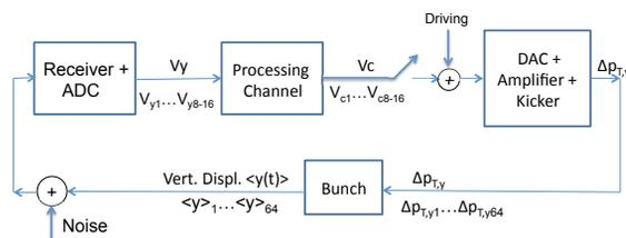
Figure 5: Block diagram of the feedback system implemented in the macro-particle code simulation.
