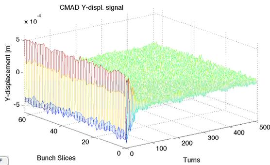
Figure 8: Vertical displacement of the multiple slices of a bunch
