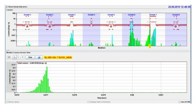
Figure 3: Beam loss pattern as recorded by the LHC Post-Mortem system indicating the loss distribution and the time profile of the loss at the BLM that triggered the beam dump.
