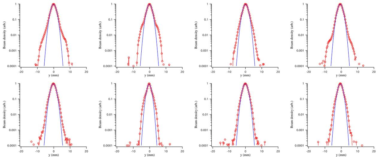
Figure 3: The vertical beam profile measured at the exit of SDTL before (upper row) and after (lower row) the buncher tuning.
