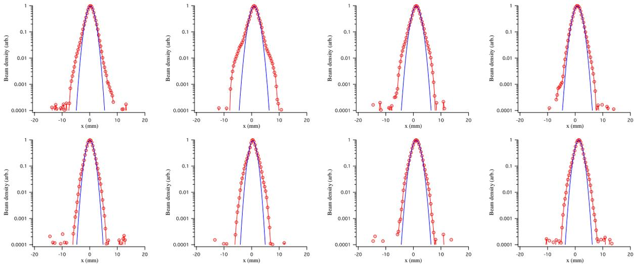
Figure 2: The horizontal beam profile measured at the exit of SDTL before (upper row) and after (lower row) the buncher tuning. There are four wire scanner profile monitors periodically placed after SDTL, and each column corresponds to the measurement result obtained with each monitor. Red circle: measurement, blue line: Gaussian fit. The same notation is adopted in Fig. 3.
