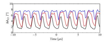
Figure 7: Phase error between 10 and 20 MHz versus time (LHC50ns,  $1.9 \cdot 10^{11}$  ppb, constant offsets removed). The vertical scale is in degrees with respect to the lower harmonic h = 21. The batch length is 12 (black), 24 (red) or 36 bunches (blue), corresponding to 2/7, 4/7 and 6/7 of the circumference. The periodicity is  $1/f_{\rm rev} = 2.1 \,\mu$ s.
