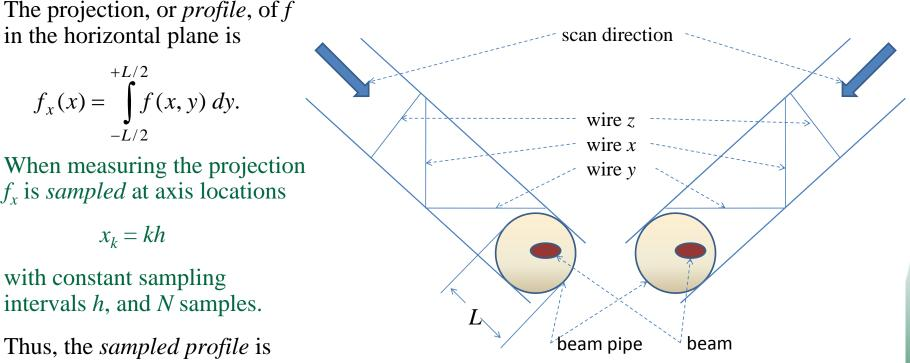
Prototypical Profile Device – The Wire Scanner
