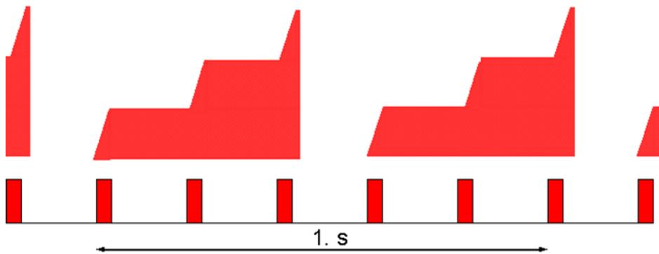
8 GeV Linac: 1ms pulses at 5Hz
