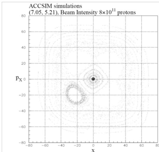
Figure 4: ACCSIM simulation of the  $x - p_x$  phase space plots of 20 test particles when the horizontal tune was 7.05 and the injection beam intensity was  $8 \times 10^{11}$  protons.
