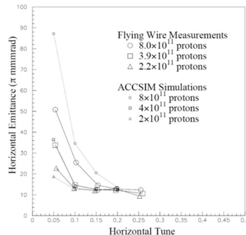
Figure 6: ACCSIM results of the horizontal 87% emittance as a function of the horizontal tune are shown in small symbols and dotted lines. Flyingwire measurement results are shown in large symbols and solid lines.
