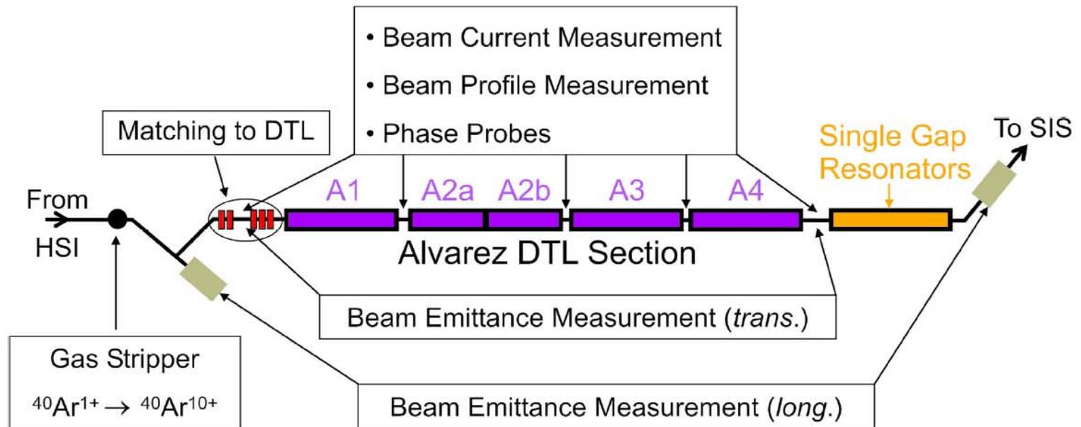
Figure 2.1: Schematic set-up of the experiments.
