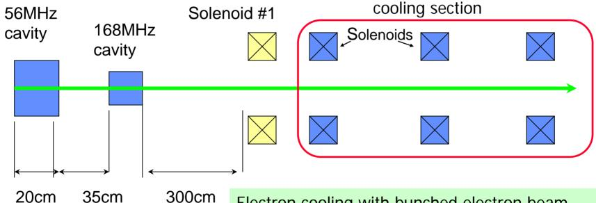
Electron cooling with bunched electron beam produced by 56MHz cavity – long bunch is needed to minimize space-charge effect in beam transport at low-energies.
